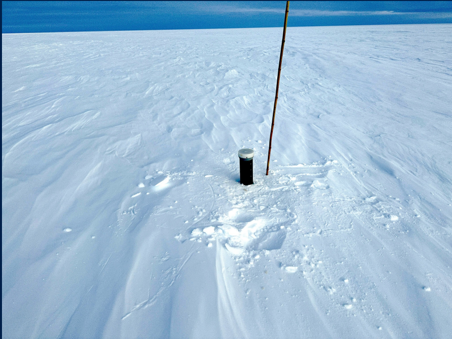
Communication penetrator on Antarctica 100 km away from Syowa station.
