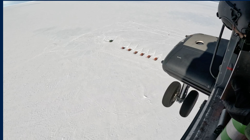
Penetrator drop test from 120 m height on Antarctica. The penetrator penetrated vertically.
