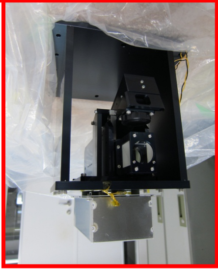
Echelle grating drive mechanism
