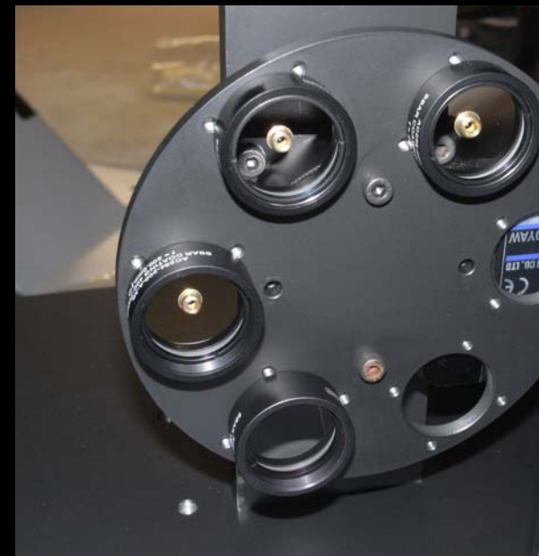
Fig. Occulting masks in the turret
