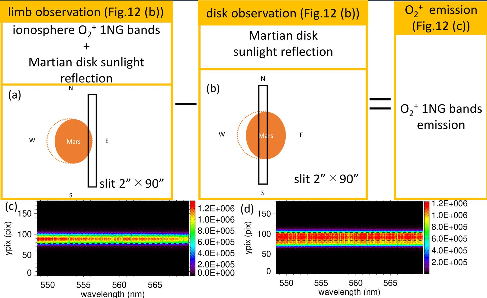
Fig.11 (a, b): Schematic view of the observing slit geometry (a) observation of Martian disk (b) observation of Martian limb. (c, d): The spectrum image of (c) limb, and (d) disk.
